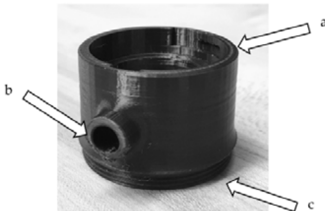
Figure 8 Isolated photo of final coupler prototype (2017). Key design features: K4b2 connection interface (a), press-fit air sampling port (b), and the TrueOne 2400 threaded-interface (c).
