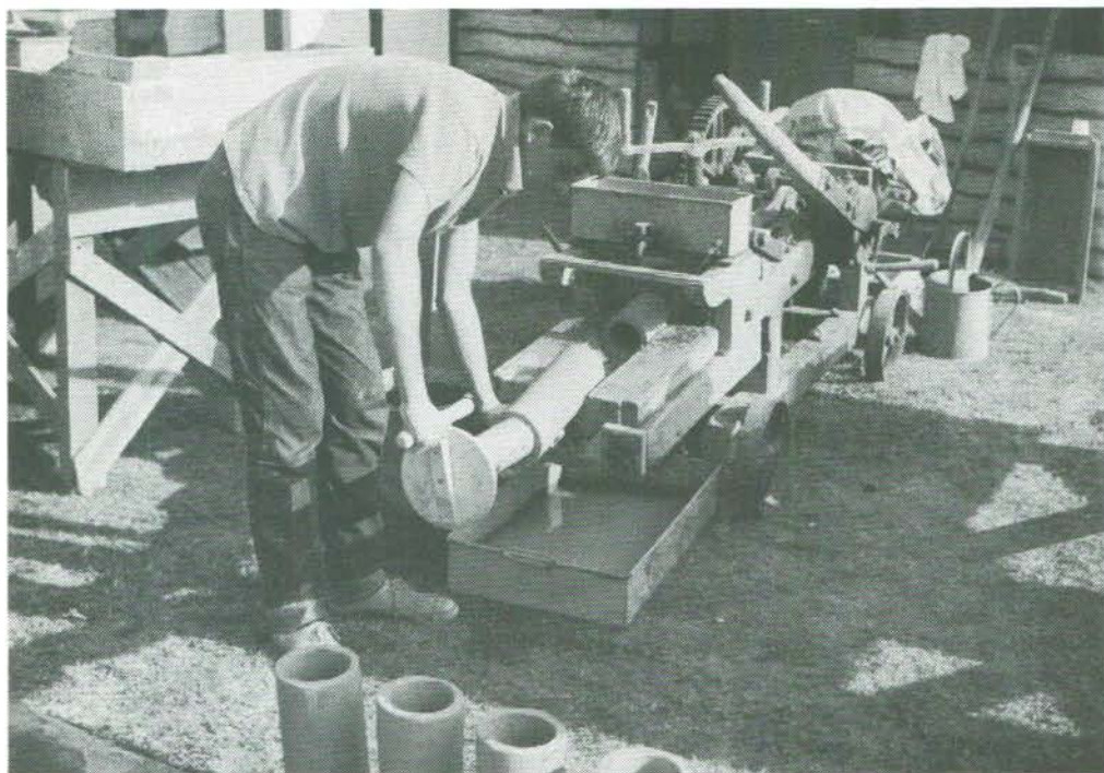
Machine for the production of land drainage pipes — mid-nineteenth century used at Ashburnham Brickworks, Battle, Sussex. (John Upton).
