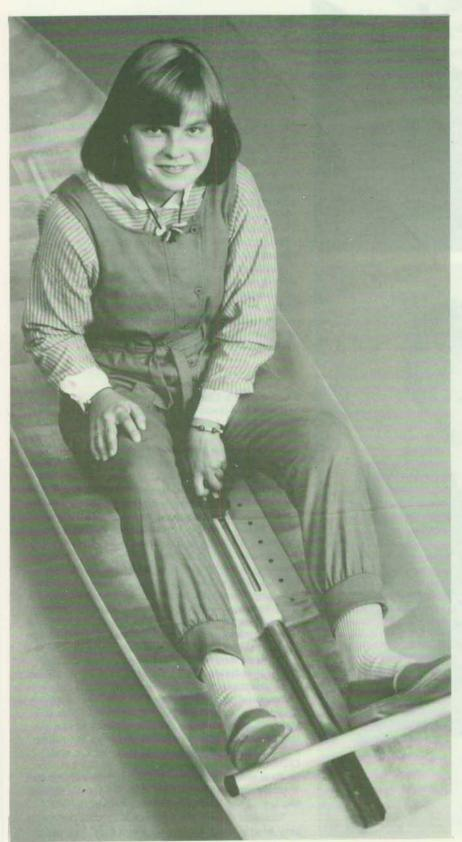
advantage is that adjustments can be made while the canoeist is in position, so that the most comfortable leg length can be fixed quickly and easily for each person.
