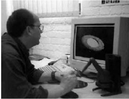
Figure 5: The SensAble FreeForm/Phantom haptic feedback device.
