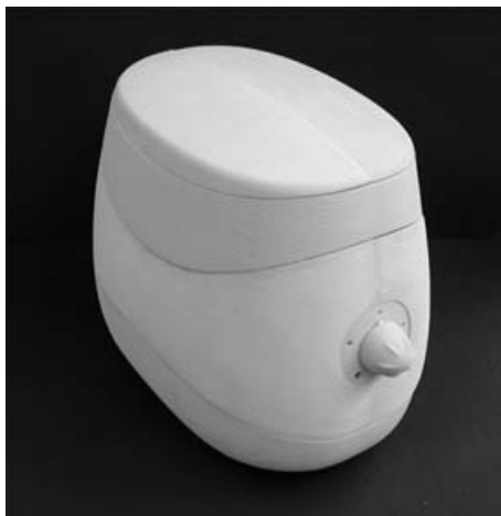
Figure 13: Z-Corporation concept model produced using FreeForm/Phantom geometry.
