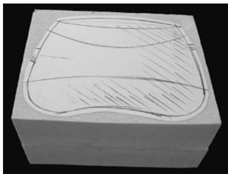
Figure 6: Orthographic sketches bonded onto Styrofoam block.
