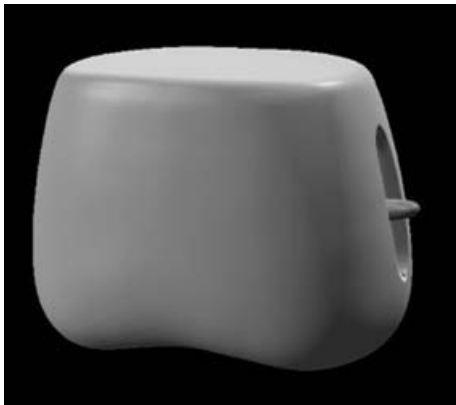
Figure 12: Final form defined using CAD-type functionality of FreeForm/Phantom, not haptic interaction.
