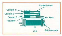
Figure 8: Operating principle of a relay.
