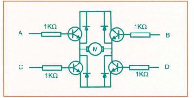
Figure 12: PIC codes supplied to transistor bases for controlling motors.
