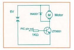
Figure 4: Measuring the trigger voltage for a Darlington Pair arrangement.
