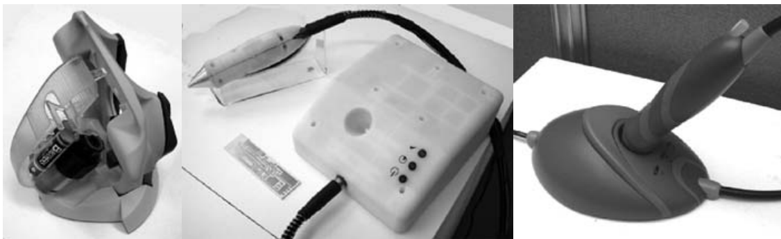
Figure 2: A range of CNC and RP manufactured prototype parts
