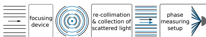
FIG. 1 Basic layout of a phase shift experiment with a single atom and a coherent beam. For further explanations see text.
