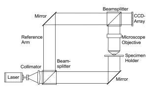
FIG. 1 Typical arrangement for digital holographic microscopy.
