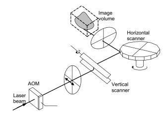
FIG. 10 Schematics of MIT's Mark I holographic display.
