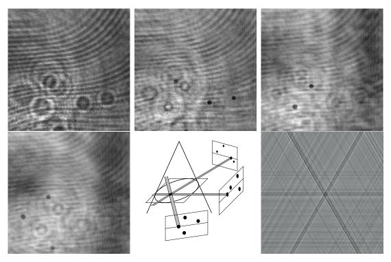
FIG. 6 Digital hologram of particle field (a), reconstructed intensities (b), (c), (d), tomography geometry (e), reconstructed plane using filtered backprojection (f)
