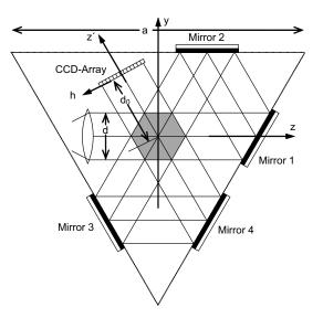
FIG. 4 Three-pass in-line arrangement for digital holographic particle analysis.
