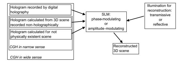
FIG. 9 Optical reconstruction of 3D scenes from digital holograms.
