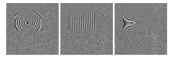
FIG. 7 Interference phase distributions of aluminum plate a) pressed from back side, b) shifted laterally, c) pressed and shifted
