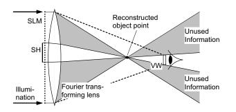
FIG. 11 Sub-hologram (SH) and virtual window (VW) in the SeeReal-concept.
