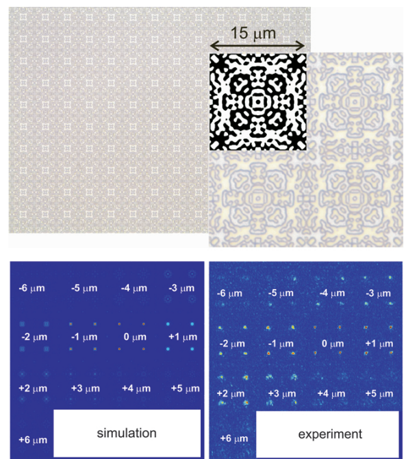
FIG. 4 Top: Microscopic image of realized binary phase structures for generating spot arrays, and the original design superimposed on the inset. Bottom: Through focus images of a subset of four spots according to simulation (left) and experiment (right).
