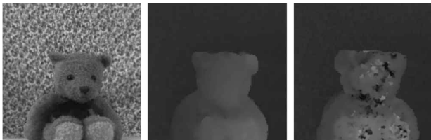
FIG. 19 Comparison of estimation results: perspective reprojected image of the real camera (left), estimation result by the proposed method (center), and estimation result by a two-view stereo method (right).
