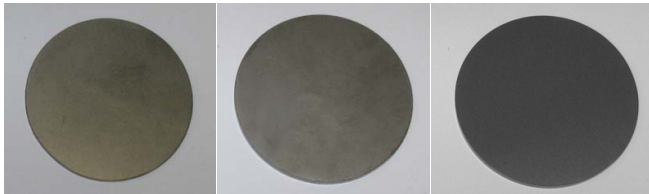
FIG. 1 Prepared samples. From left to right: ZrC, ZrB 2 , SiC pellets. The diameter of all specimens is 40 mm.
