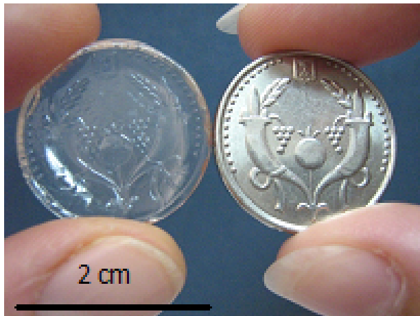
FIG. 2a Replica (left) of metal coin (right) with UV-cured fast sol-gel material manufactured by soft lithography with UV-curing process.
