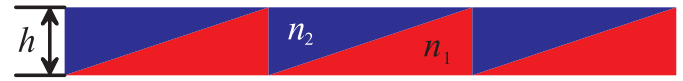
FIG. 3 Schematic representation of a DOE with common depth h , where the air between the sawtooths of a conventional blaze profile is substituted by a second material with another dispersion n_2(\lambda) .
