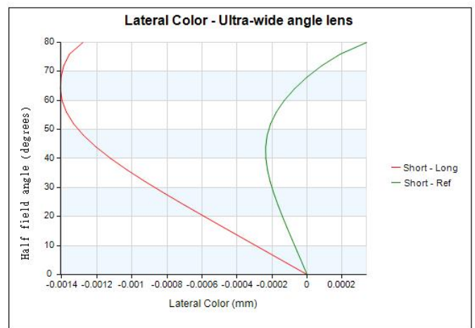
FIG. 8 Lateral color for the ultra-wide angle lens design.
