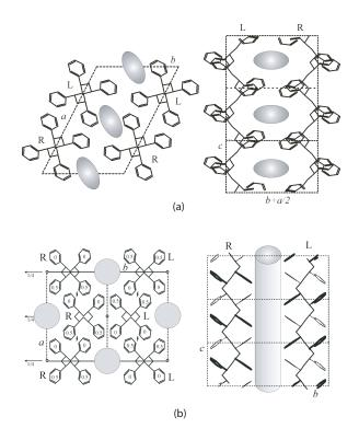
FIG. 1 Packing models of the nanoporous (a)  $\delta$  and (b)  $\varepsilon$  crystalline forms of sPS (left: up view, right: lateral view).
