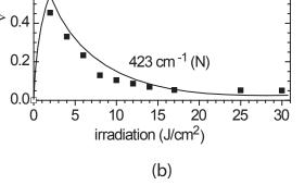
FIG. 6 (a) FTIR spectra for the range 1270-1190 cm<sup>-1</sup>, of a sPS film with a clathrate phase containing N, and after subsequent UV (254 nm) irradiation doses. (b) Photoi-somerization kinetics of N to Q, as shown by the absorbance variations of the 423 and 1237 cm<sup>-1</sup> peaks.
