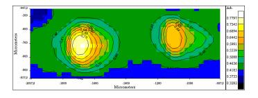
FIG. 8 FTIR of a sPS/N co-crystal film, UV irradiated in the presence of a metal mask relative to the distribution of Q molecules.
