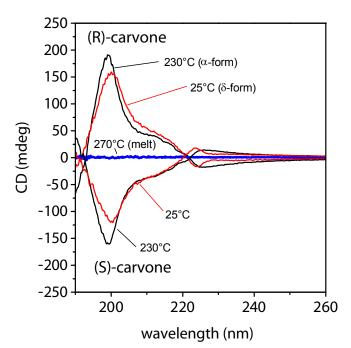
FIG. 11 Room temperature CD spectra of sPS films spin-coated at 1600 rpm from 0.25 wt% chloroform solution onto quartz surface after: (red lines) exposure to vapors of R or S-carvone; (black lines) exposure to R or S-carvone followed by thermal treatment at 230°C, leading to crystal-crystal transition from helical toward transplanar crystalline phase; (blue lines) exposure to R or S-carvone followed by thermal treatment at 270°C, leading to crystal melting.
