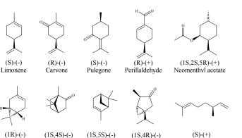
FIG. 10 Enantiomers inducing positive ICD effect in spin-coated sPS films.
