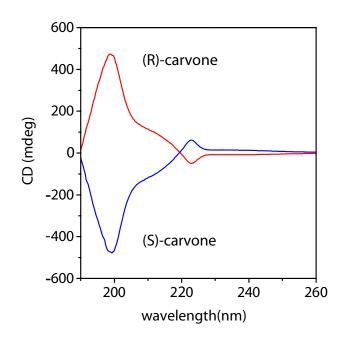
FIG. 9 CD spectra of spin-coated sPS films onto quartz surface, after exposure to vapors of (R)- or (S)-carvone. The spin-coating process has been conducted with 1 wt% chloroform solutions onto quartz surface at the spin-rate of 1600 rpm.
