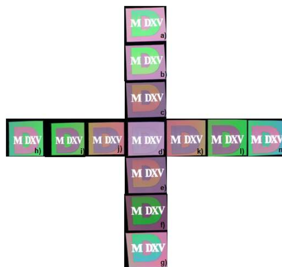
FIG. 7 Sample in movement with the vertical stripe from (a) to (g) presents the “D” in collinear incidence ( \Phi = 0^\circ ) and the rectangular area in conical incidence ( \Phi = 90^\circ ), (a) \theta = -30^\circ , (b) \theta = -20^\circ , (c) \theta = -10^\circ , (d) \theta = 0^\circ , (e) \theta = 10^\circ , (f) \theta = 20^\circ , (g) \theta = 30^\circ . With the horizontal stripe from (h) to (m) presents the “D” in conical incidence ( \Phi = 0^\circ ) and the rectangular area in collinear incidence (with \Phi = 90^\circ ), (h) \theta = -30^\circ , (i) \theta = -20^\circ , (j) \theta = -10^\circ , (k) \theta = 10^\circ , (l) \theta = 20^\circ , (m) \theta = 30^\circ . The letters “MDXV” are transparent without any metallic layers.
