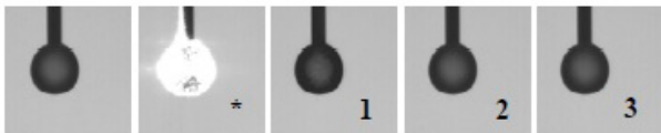
FIG. 27 Recording of the effects produced at resonant interaction on the droplet containing R6G at 10^{-3}M in distilled water by the laser beam sent in its equatorial plane and focused in its centre (position 1 Figure 2). E_1 = 0.25 mJ Movie-22 (4,9 MB).
