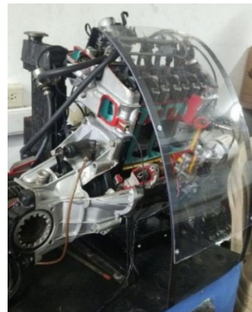
Figure 4. Cut model of an automotive powertrain. Source: own elaboration.
