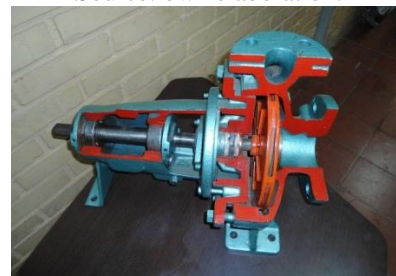
Figure 5. Cut section model of a hydraulic pump. Source: own elaboration.
