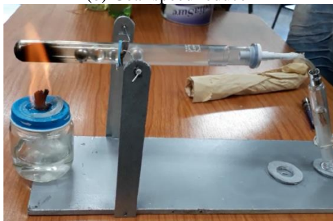
(c) Marble type Stirling engine
