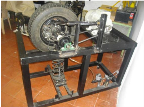
Figure 6. Model of a quarter of vehicle. Source: own elaboration.
