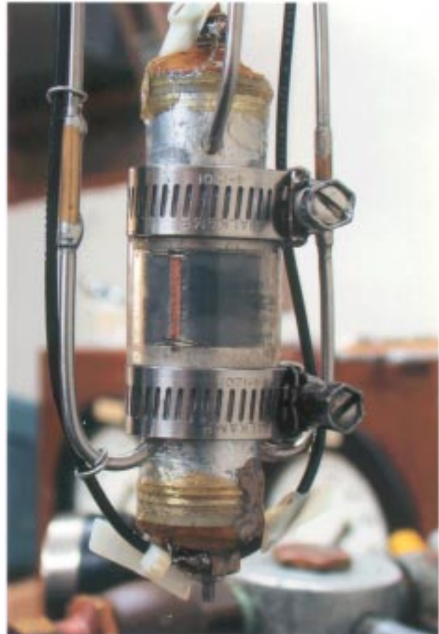
FIGURE 4. Assembly of a coal sample in the vinyl sleeve, and transducers on both sides. Notice the tubes to apply pore pressure with methane. Also, a copper braid is observed on the side of the coal sample. This copper braid facilitates the gas saturation of the coal sample.
