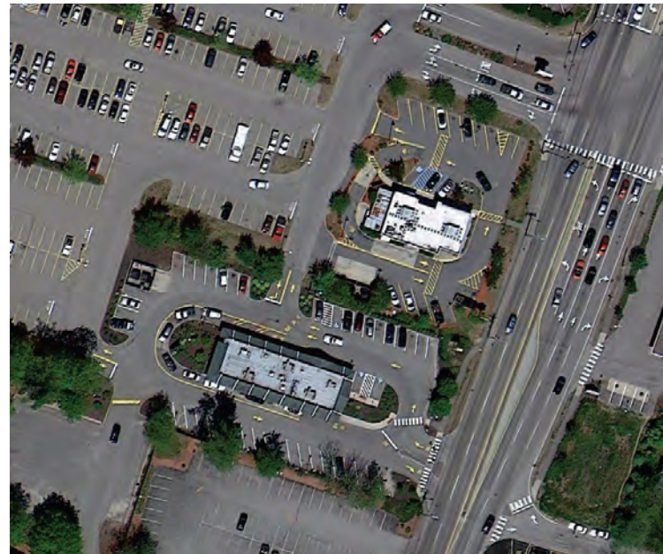
Figure 4-10: Interconnected parking lots in Saco, Maine
