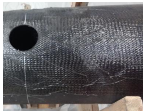
Figure 7: Acceptable wrinkling in the resin layer of a BiaB FRP tube
