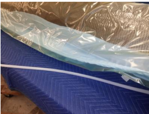
Figure 6: Bagging film wrinkles acceptable in the resin layer of a BiaB FRP tube
