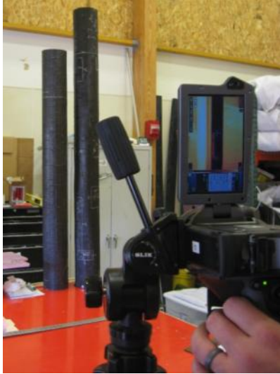
Figure 13: Infrared camera in use
