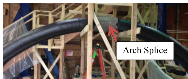
Figure 12: Key inspection location, spliced arch in laboratory
