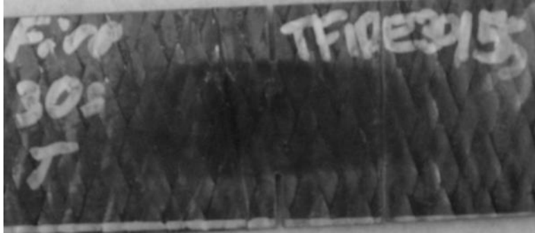
Figure 8: Fibers exposed due to fire damage
