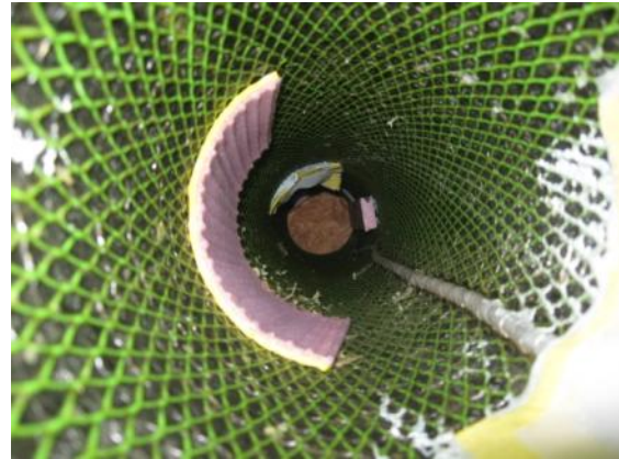
Figure 15: Inside of tube with artificial voids
