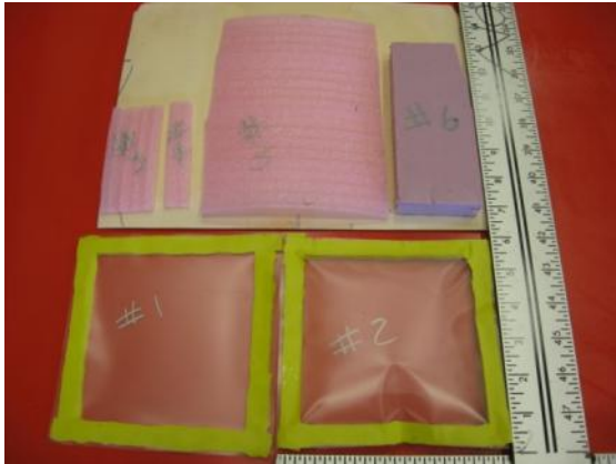
Figure 14: Materials used to create artificial voids
