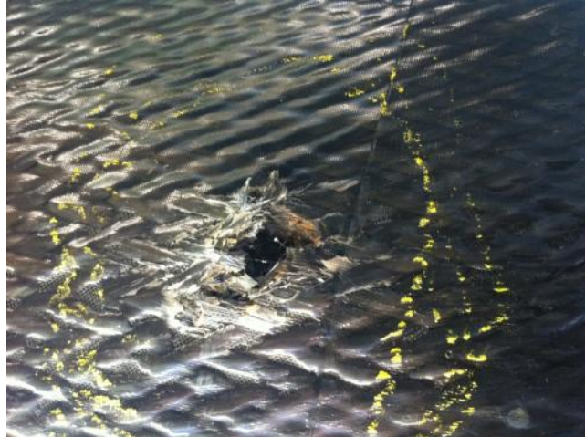
Figure 5: Full puncture/hole in carbon fiber laminate
