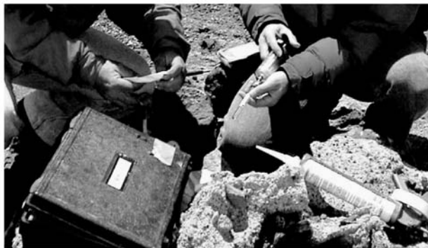
FIGURE 3. a) Example of radon and CO 2 in soil station deployment, used in this study. b) collecting data.
