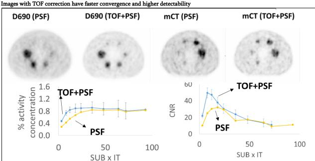
Spheres with TOF correction converge faster than non-TOF images. The quantitative accuracy at convergence, however, is not strongly affected. The curves shown above were calculated for the 37mm sphere. TOF corrections also improve detectability. The curves were calculated for GE D690. The images were reconstructed at 18 SUB×IT with 6.4mm filtration for D690 and 21 SUB×IT with 5mm filtration for mCT.
