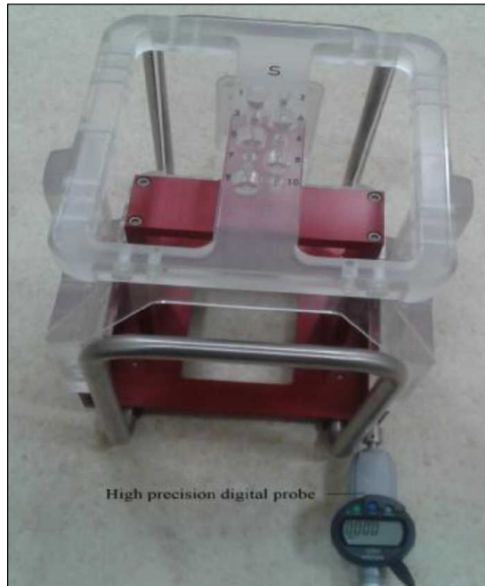
Figure 2: Repositioning check tool (RCT) and calibration of electronic digital probe.
