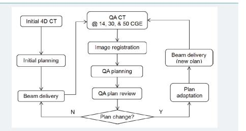
Figure 1: A clinical workflow of adaptive planning for lung cancer treatment using uniform scanning proton therapy (from Zheng [15]).
