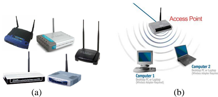
Gambar 9. Wireless Access Point
