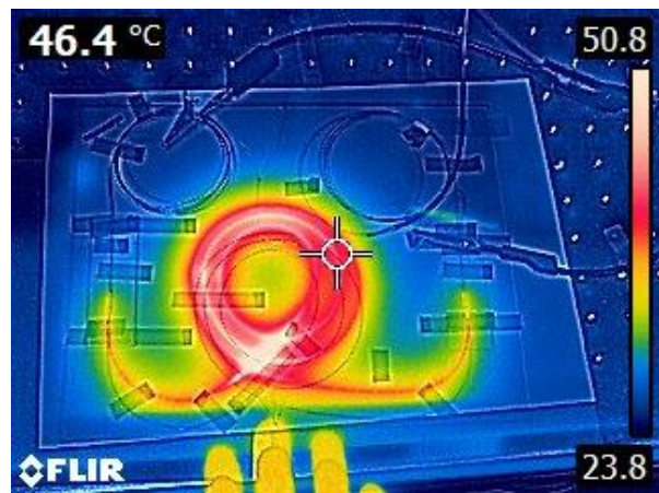
Fig. 4. Thermal infrared image of the optical fiber segment employed in the test while DC current produces Joule heating on its carbon coating.
