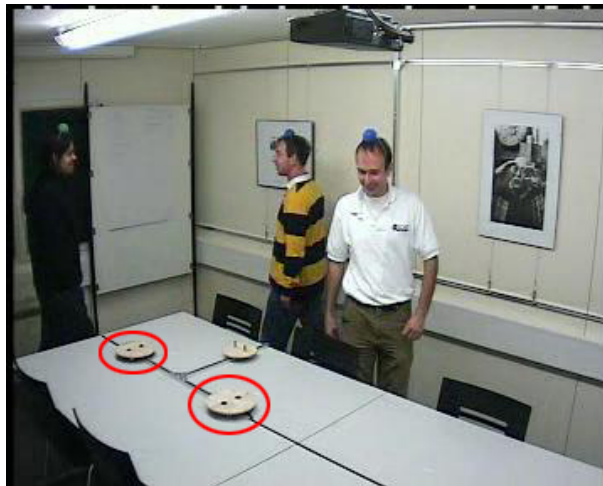
Figure 1.1: Example of a multimodal localization system [1]. Note that the red circles shows where the microphone arrays are located.
