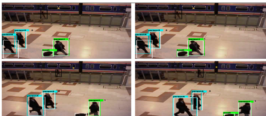
Figure 4.7: From PETS2006 S1-T1-C3 clip, we have seen that YOLO struggles to detect backpacks and suitcases much more than with the GBA dataset.
