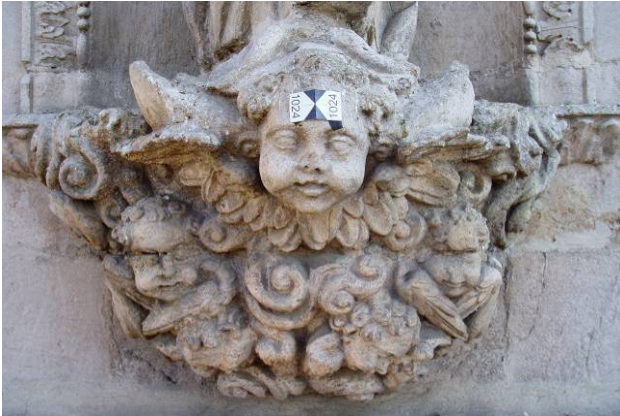
Fig. 5. Type of targets used for control points
