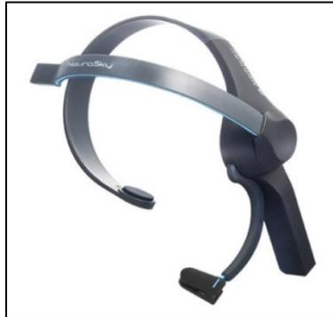
Figura 5.1 Casco Mindwave mobile [9]
