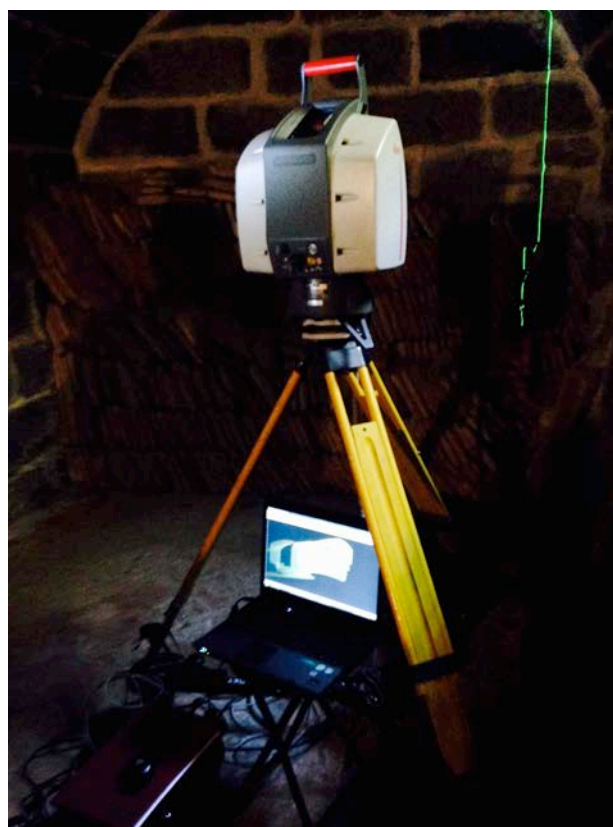
Figure 8. The laser scanner surveying the upper spaces.
