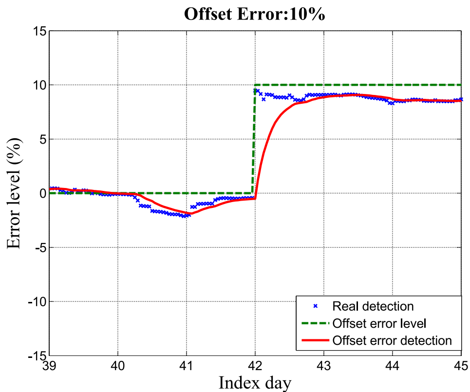
Figure 4.15: CT 50001 - Gain 0% & Offset 10%: Detecting 0% gain and 10% offset errors during the days after training.
