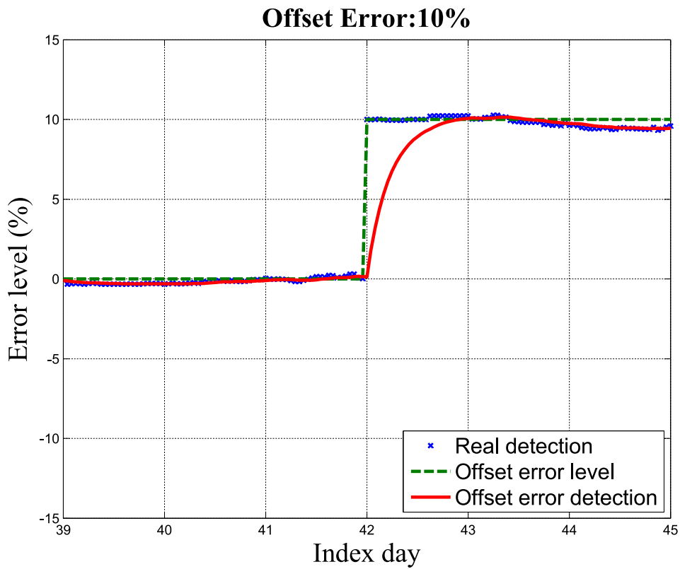
Figure 4.7: CT 1779 - Gain 0% & Offset 10%: Detecting 0% gain and 10% offset errors during the days after training.
