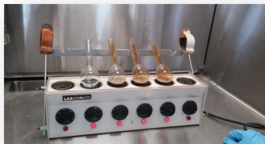
Fig. 16 Digestion of soils with nitric and perchloric acid.
