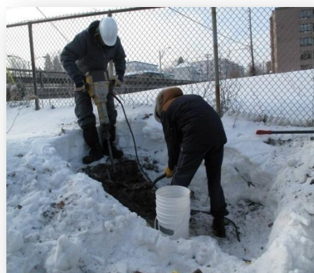
Fig. 5 Removal of snow, capping and soil storing in plastic cubes in sampling.
