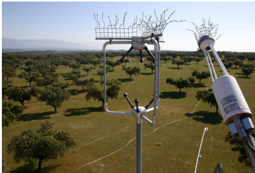
Figure 11. Picture from top of the EC system showing the setup of the sonic anemometer and the open path analyzer. Wiring on top was installed to avoid the birds to place on top of the instruments.
