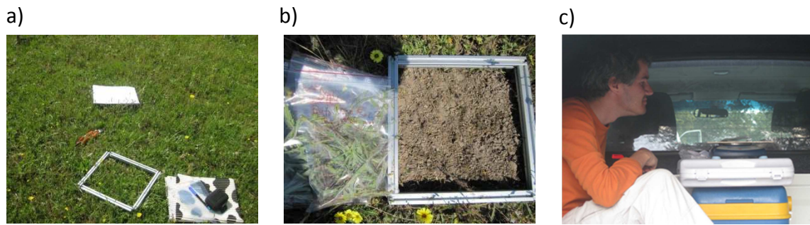
Figure 9. a) Field instrumentation consisting on a 25x25 cm quadrant, clippers, field notebook, zip plastic bags and pen. b) Picture of a frame after the sample has been collected and kept in the zip bag. c) Weighting of collected samples in the field in the trunk of the car to avoid wind during the weighting process.
