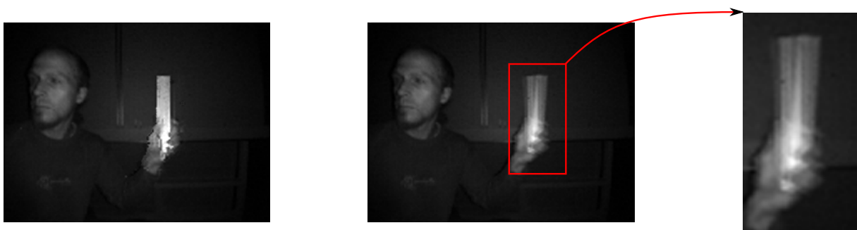
Figure 1.3: Motion artifacts phenomenon. We show a planar object moving in a perpendicular direction in front of the camera. On the left, we show the original object. On the right, the captured amplitude image and a zoomed version of the affected area, respectively.
