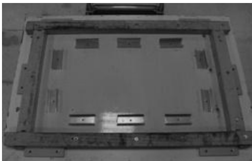
Figure 3a: Kraai Slab Test
