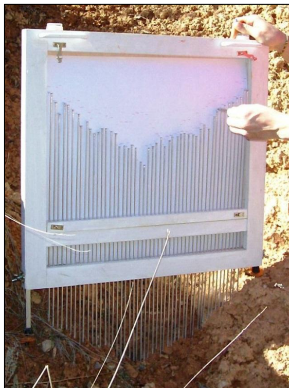
Fig. 3.1.6. Measurement of rill erosion with a needle micro-profiler.
