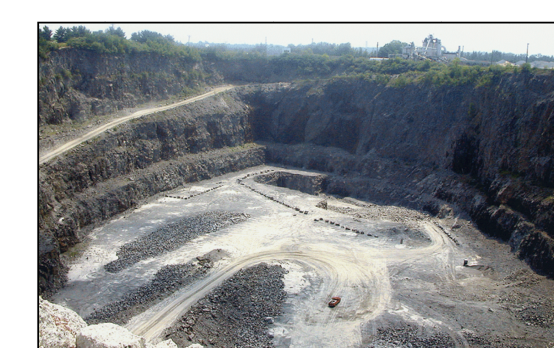
Photo 8. Blue Rock quarry between Westbrook and Portland. Biotite granofels of the Berwick Formation is quarried here for crushed rock aggregate. The Maine Turnpike is just out of sight on the left side of the photograph.
