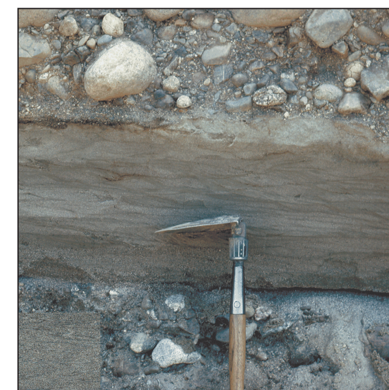
Gravel over sand over gravel: p-es/p-c -- Close-up of pit face showing intertidal(?) sand unit between pebble-cobble gravel beds in upper part of glaciomarine delta, Columbia Falls.
