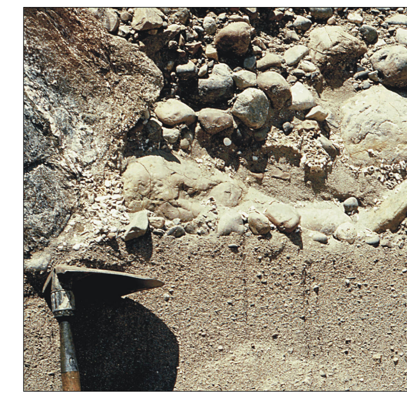
Pebble to boulder gravel (fossiliferous) over gravelly sand: p-b/ds -- Close-up of pit face in marine nearshore deposit with fossil shells and barnacle-encrusted stones.
