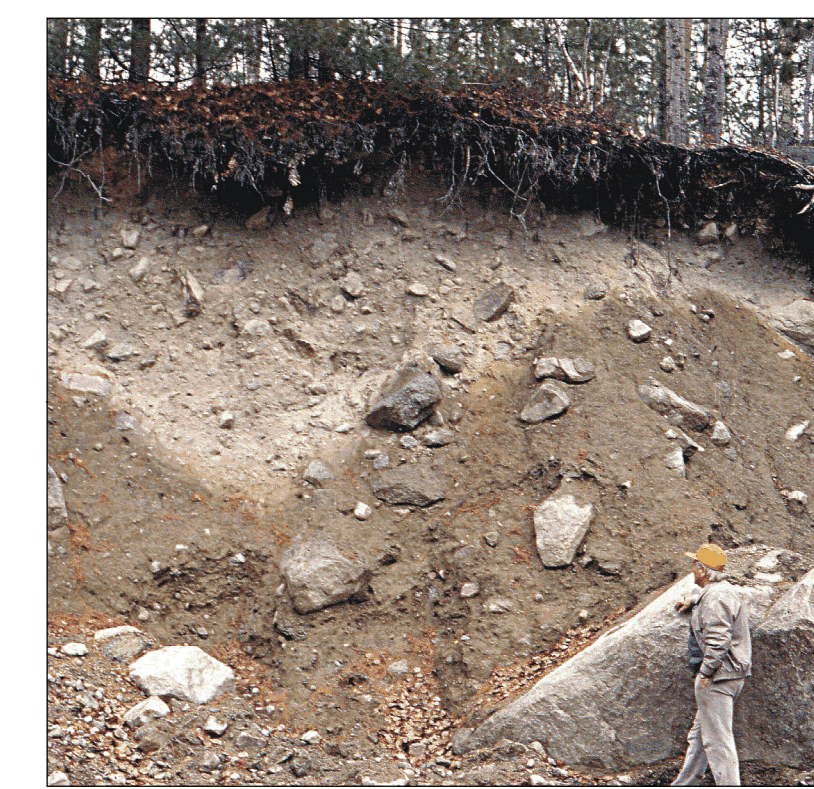
Till: d(t) -- Borrow pit near Millinocket, exposing sandy, bouldery till. This stony till commonly occurs in areas of granitic bedrock.
