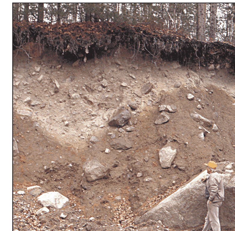
Till: ds(t) -- Borrow pit near Millinocket, exposing sandy, bouldery till. This stony till commonly occurs in areas of granitic bedrock.
