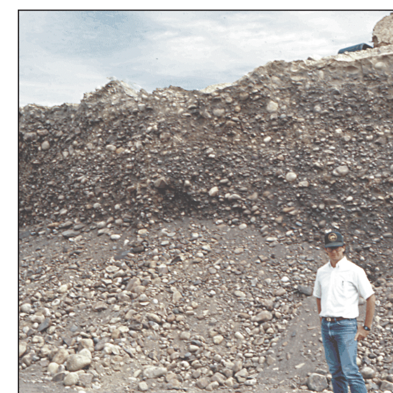
Pebble to cobble gravel: p-c -- Pit in upper part of glaciomarine delta in Norridgecock, Kennebec River valley, showing massive gravel deposited by meltwater streams flowing across delta top.
