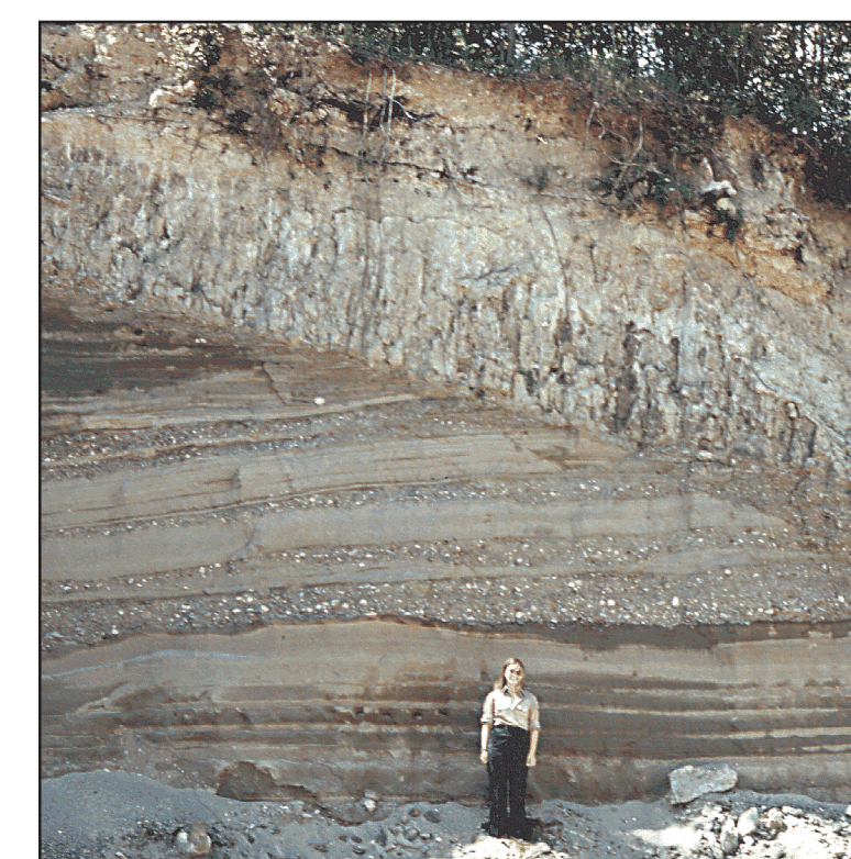
Clayey silt over sand with pebble-cobble gravel: st,cy/s,p,c -- Borrow pit in Kennebec River valley, Pittston, showing glaciomarine sea-floor mud (Presumpscot Formation) overlying sand and gravel deposited in submarine fan at glacier margin.
