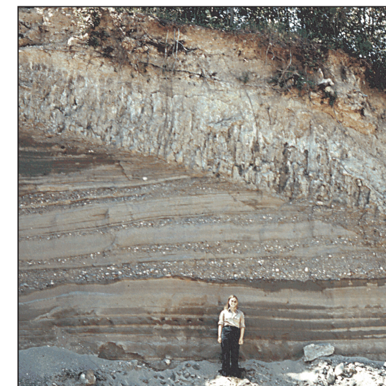
Clayey silt over sand with pebble-cobble gravel: st, cy/s, p, c -- Borrow pit in Kennebec River valley, Pittston, showing glaciomarine sea-floor mud (Presumpscot Formation) overlying sandy and gravel deposited in submarine fan at glacier margin.
