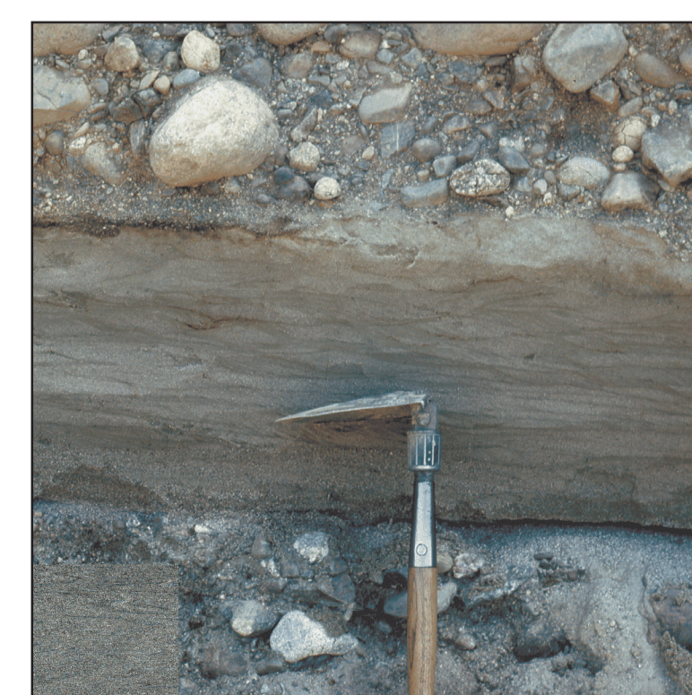
Gravel over sand over gravel: p-cs/p-c -- Close-up of pit face between pebble-cobble gravel beds in upper part of glaciomarine delta, Columbia Falls.
