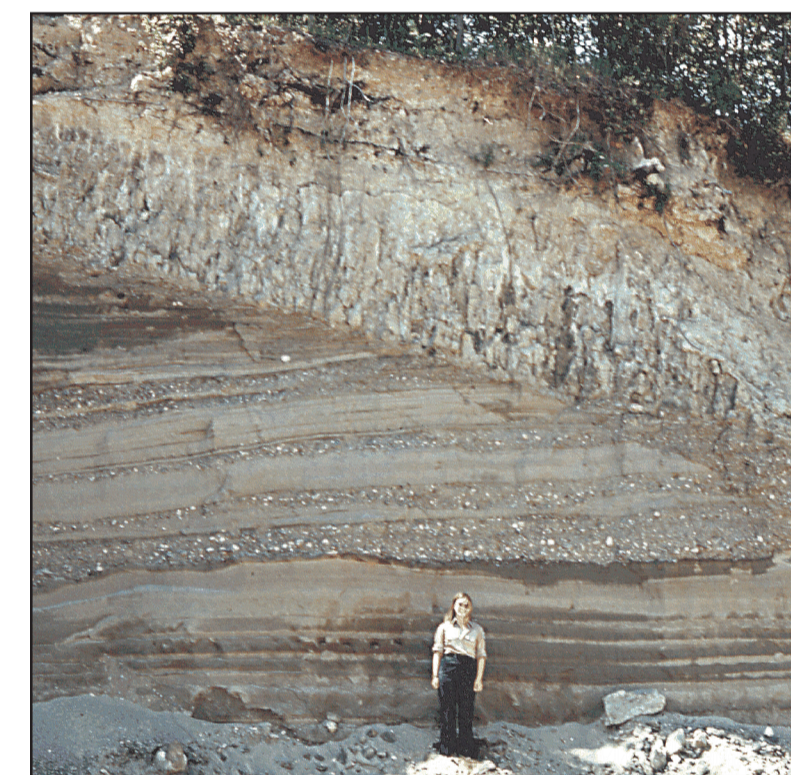
Clayey silt over sand with pebble-cobble gravel: st/cy/s,p,c -- Borrow pit in Kennebec River valley, Pittston, showing glaciomarine sea-floor mud (Presumpscot Formation) overlying sand and gravel deposited in submarine fan at glacial margin.
