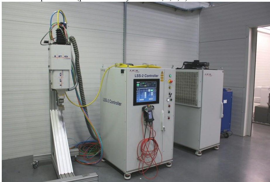
Figure 3. The view of the Laser SEAM Stepper welding station
