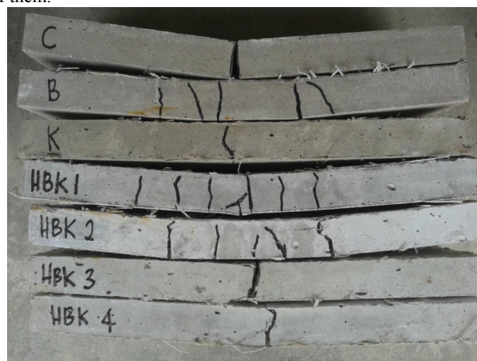
Figure 6. Crack pattern of test panels cured in cyclic exposure.
