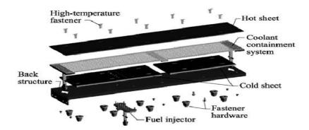
Figure 8 Exploded view of the cooling structure consisting of C / SiC composite panels and Ni alloy tubes
