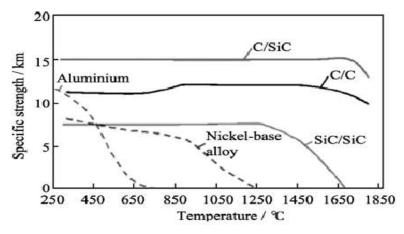
Figure 6 Ratio of strength to weight as a function of temperature
